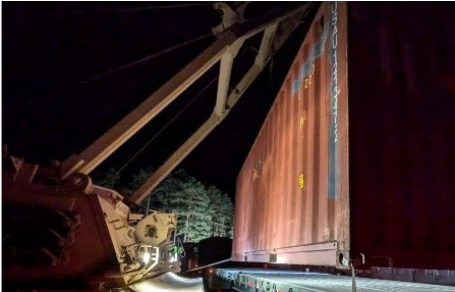
Figure 3: M88A3 loading a container onto a trailer. Note the safety guide cables on the lower corners. (Photo by author)
